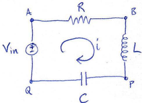
Current flows clockwise because it flows from "+" terminal of voltage source to "-" terminal.
